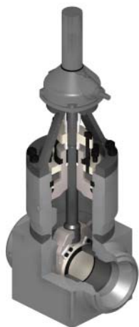
An example: 14" F91 gate manual gear operated, design temperature: 590°C design pressure: 276 bar (intermediate between 2500# and 4500#)
