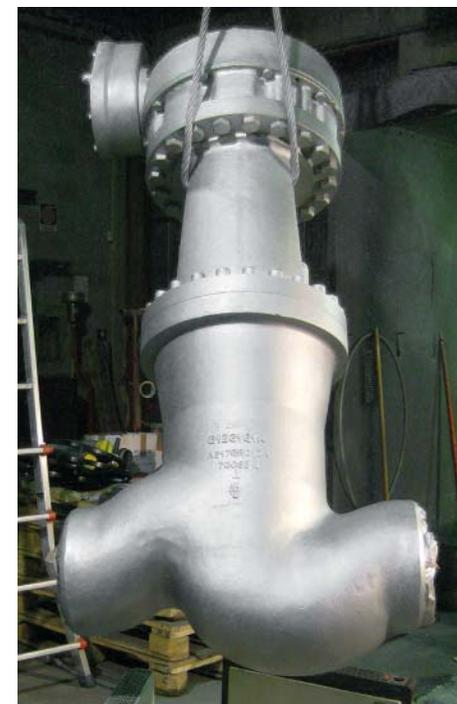
A typical example are class-1500 ASME valves, which are normally supplied according to this dimensional table. Other dimensions and pressure classes available as per customer request.
