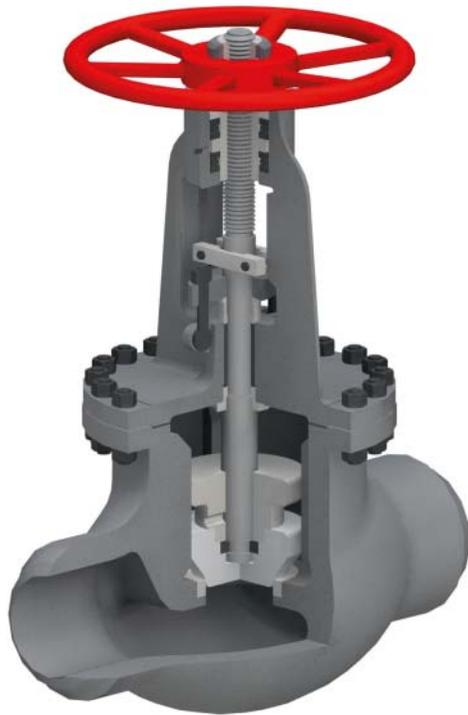
FLUITEK ORSENIGO VALVES has a very extended experience in globe valves manufacturing. In this kind of valve, the disc is moving in a perpendicular direction away from the seats. This implies the disc-to-seat ring contact to be at right angle, which permits the force of closing to tightly seat the disc, reducing the seat leakages. Normally, the globe valves are arranged so that the disc closes against the direction of fluid flow.
