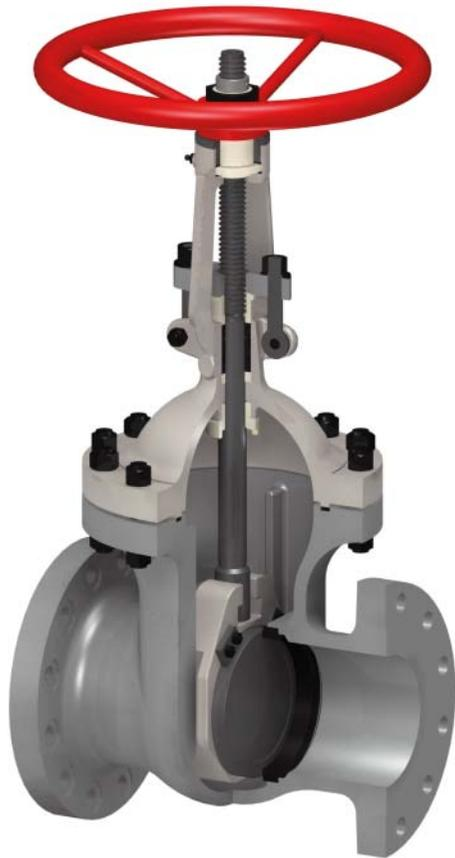
This type of on-off valve is an alternative to the traditional wedge type gate valves. The disc is in two halves, spring loaded, that seat on parallel seat rings. The disc “slides” in contact with the seats, hence the name. The advantages of this product versus the traditional wedge type product are:
