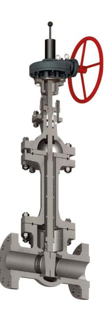
Bellows seal valves are used in applications where a hermetic tightness is essential in order to prevent any possible leakage of process fluid into the atmosphere, where the fluid is particularly hazardous (poisonous, aggressive, radioactive). FLUITEK ORSENIGO VALVES is specialised in gate valves with bellows seals, in particular in the manufacturing ٥f٠
